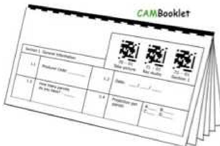
Figure 7.8: Final design of the inspection booklet. Compact, laminated, rain and dirt-proof design allows inspectors to enter data directly on the phone, including relevant images and audio.
