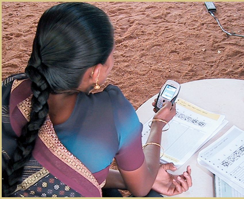
Figure 2. A prospective user entering CamForm data using the mobile phone's alphanumeric keypad.
