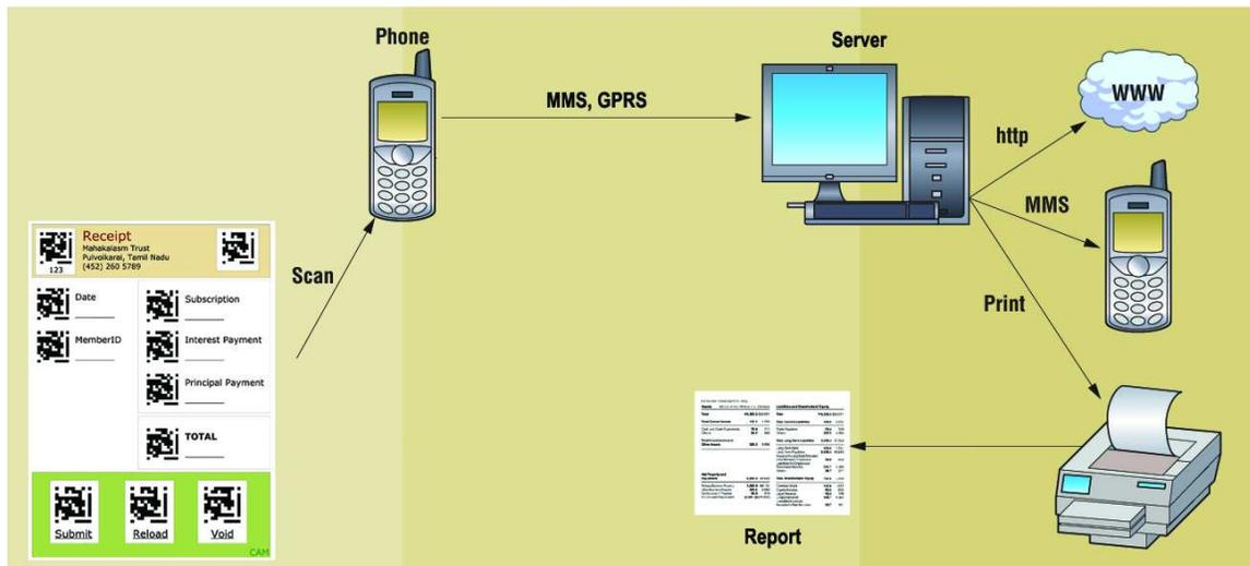
Figure 4.1: Three-tiered CAM framework. CAM provides the appropriate information medium for each context. Rural users transfer paper-based information to roving smart-phone middleware, which uploads the data to remote storage for distribution in various ways.
