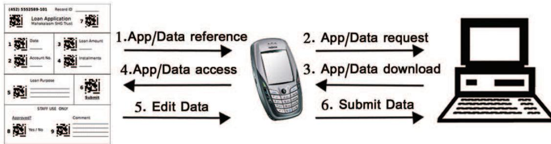
Figure 4.5: An example set of steps in accessing and using a CAM application. Except for steps 4-5, there can be arbitrary time and distance between each step, supporting an offline, asynchronous interaction model appropriate for rural areas.
